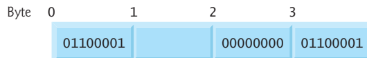
Fig. 10.1 | Possible storage alignment for a variable of type struct example showing an undefined area in memory.
