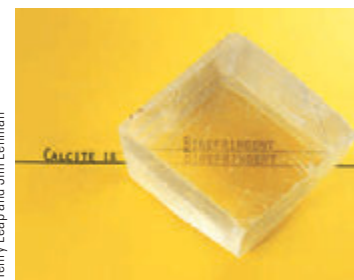
Figure 38.31 A calcite crystal produces a double image because it is a birefringent (double-refracting) material.
