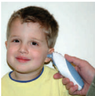
Figure 40.8 An ear thermometer measures a patient's temperature by detecting the intensity of infrared radiation leaving the eardrum.
