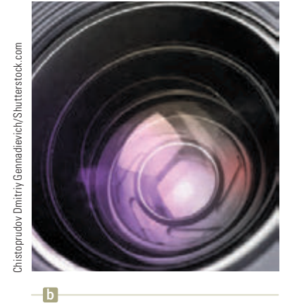
Figure 37.12 (Example 37.4) (a) Reflective losses from a silicon solar cell are minimized by coating the surface of the cell with a thin film of silicon monoxide. (b) The reflected light from a coated camera lens often has a reddish-violet appearance.
