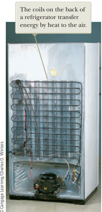
Figure 22.6 The back of a household refrigerator. The air surrounding the coils is the hot reservoir.
