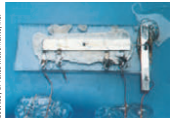
Figure 43.32 Jack Kilby’s first integrated circuit, tested on September 12, 1958.
