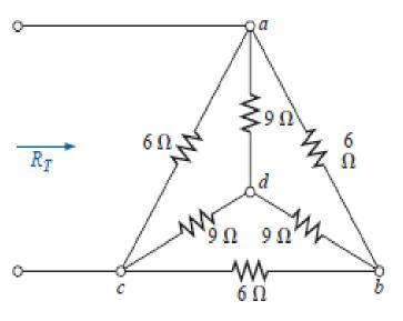
$$R_{\rm Y} = \frac{R_{\Delta}}{3} = \frac{6 \,\Omega}{3} = 2 \,\Omega$$
