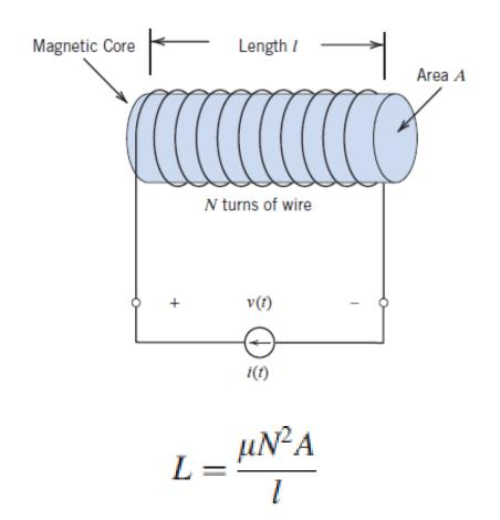
Inductor is used to store energy in electromagnetic field
