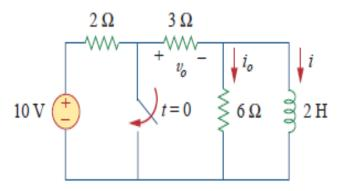
For t < 0, the switch is open. Since the inductor acts like a short circuit to dc, the 6- $\Omega$  resistor is short-circuited, so that we have the circuit shown in Fig. 7.20(a). Hence,  $i_o = 0$ , and
