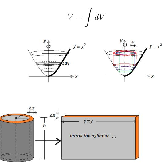
$V_{shell} = 2\pi r h \Delta x = 2\pi (\text{shell.radius}) (\text{shell.height}) \Delta x$
