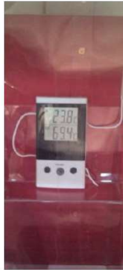
Clay Tiles + Insulator 23.8°C
