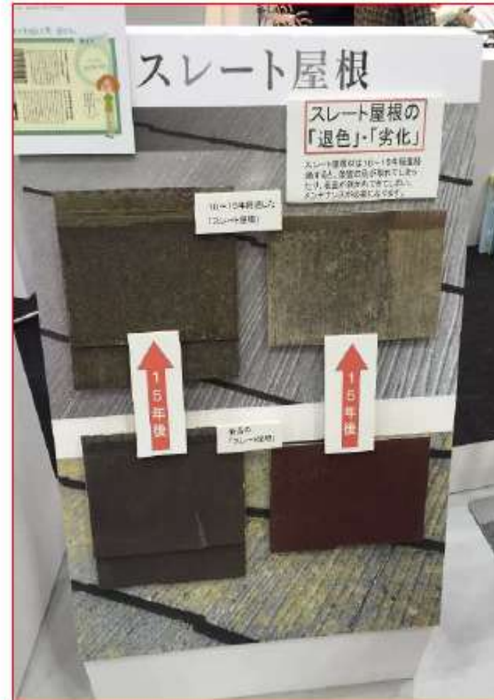
Others Roofing materials after 15 years
