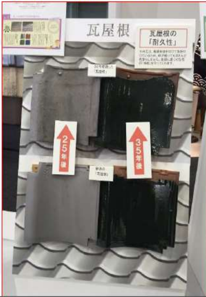
Clay Roof Tiles after 25 & 35 years
