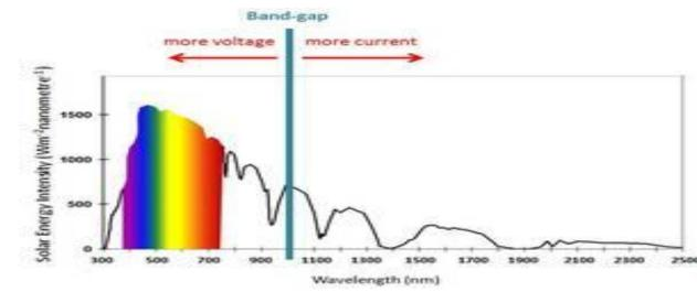
Photovoltaics Technologies For sunlight on Earth, the 'best-position' line is at <u>about 1200nm</u>, corresponding to a <u>maximum</u> <u>efficiency of about 31%.</u>
