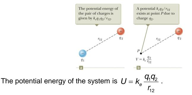
If the two charges are the same sign, U is positive and work must be done to bring the charges together.
