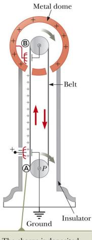
The charge is deposited on the belt at point (A) and transferred to the hollow conductor at point (B).
