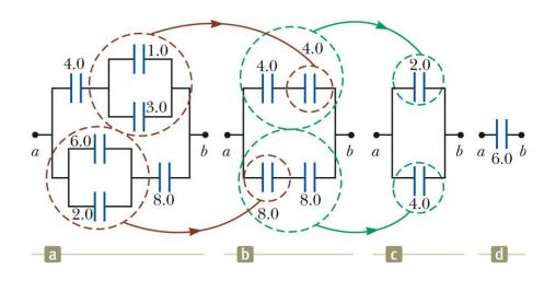
The 1.0- $\mu$ F and 3.0- $\mu$ F capacitors are in parallel as are the 6.0- $\mu$ F and 2.0- $\mu$ F capacitors.
