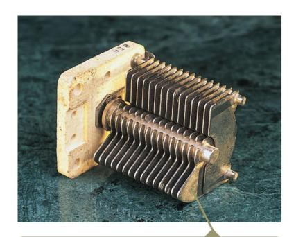
When one set of metal plates is rotated so as to lie between a fixed set of plates, the capacitance of the device changes.
