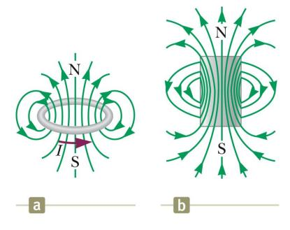
Figure (a) shows the magnetic field lines surrounding a current loop.
