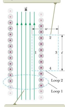
Ampère's law applied to the circular path whose plane is perpendicular to the page can be used to show that there is a weak field outside the solenoid.
