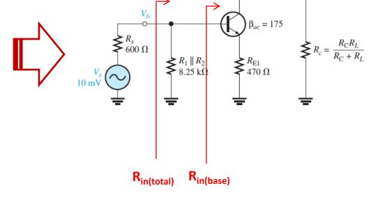
Next, determine the attenuation in the base circuit.
