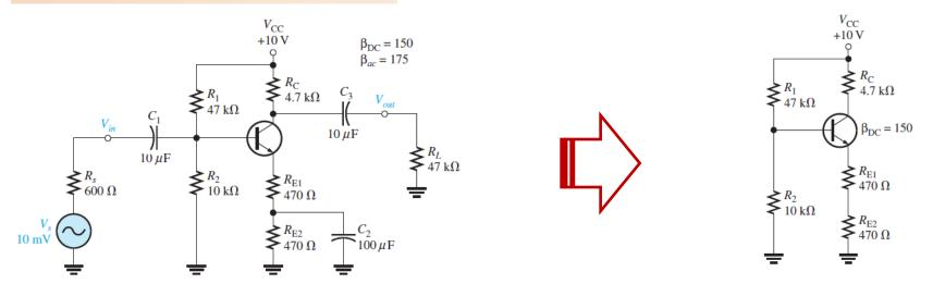
$$R_{\text{TH}} = \frac{R_1 R_2}{R_1 + R_2} = \frac{(47 \text{ k}\Omega)(10 \text{ k}\Omega)}{47 \text{ k}\Omega + 10 \text{ k}\Omega} = 8.25 \text{ k}\Omega$$
