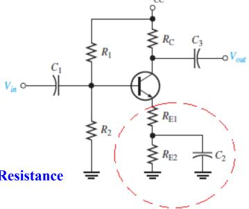
☐ The Effect of Swamping on the Amplifier's Input Resistance
