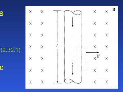
For a wire of length / caring a current / in a magnetic field with a flux density B that makes an angle  $\theta$  to the wire, the magnitude of the force is:
