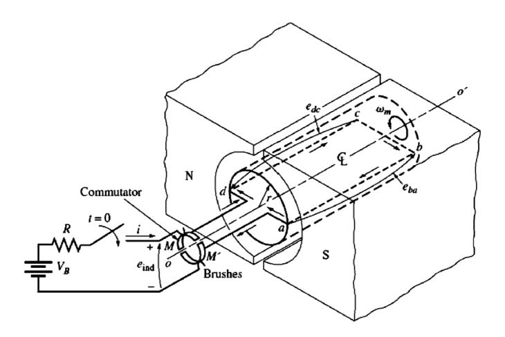
Example 8–1. Figure 8–6 shows a simple rotating loop between curved pole faces connected to a battery and a resistor through a switch. The resistor shown models the total resistance of the battery and the wire in the machine. The physical dimensions and characteristics of this machine are
