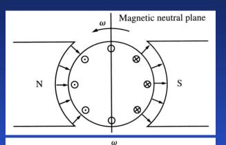
A two-pole DC machine: initially, the pole flux is uniformly distributed and the magnetic neutral plane is vertical.
