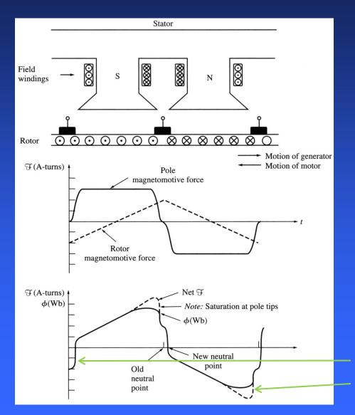
In generators, flux weakening reduces the voltage supplied by a generator.
