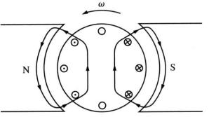
When the load is connected, a current – flowing through the rotor – will generate a magnetic field from the rotor windings.
