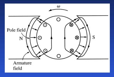
This rotor magnetic field will affect the original magnetic field from the poles. In some places under the poles, both fields will sum together, in other places, they will subtract from each other
