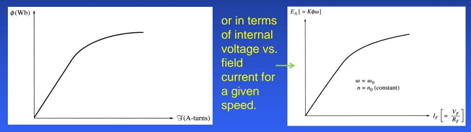
To get the maximum possible power per weight out of the machine, most motors and generators are operating near the saturation point on the magnetization curve. Therefore, when operating at full load, often a large increase in current  $I_F$  may be needed for small increases in the generated voltage  $E_A$ .
