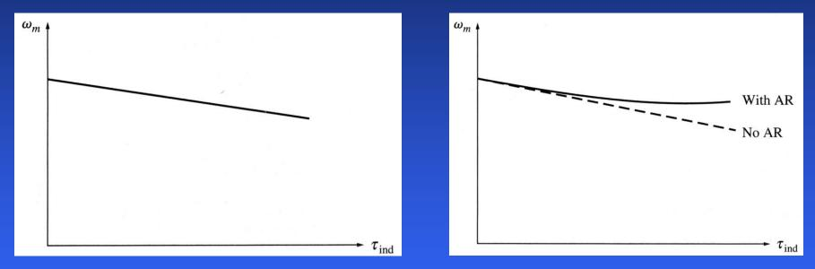
However, if a motor has an armature reaction, flux-weakening reduces the flux when torque increases. Therefore, the motor's speed will increase. If a shunt (or separately excited) motor has compensating windings, and the motor's speed and armature current are known for any value of load, it's possible to calculate the speed for any other value of load.
