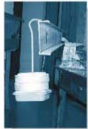
Demonstration of how a cantilever beam deflects when loaded through the centroid (above) and through the shear center (below).
