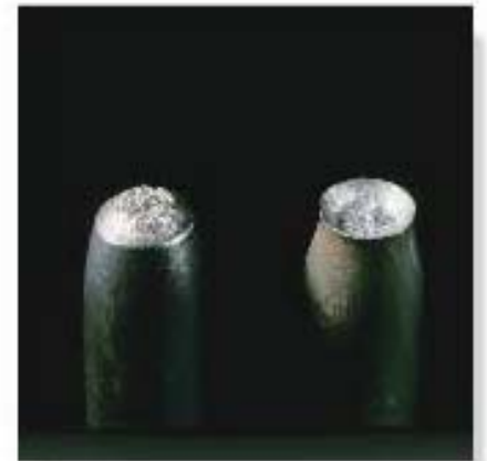
This steel specimen clearly shows the necking that occurred just before the specimen failed. This resulted in the formation of a "cup-cone" shape at the fracture location, which is characteristic of ductile materials.
