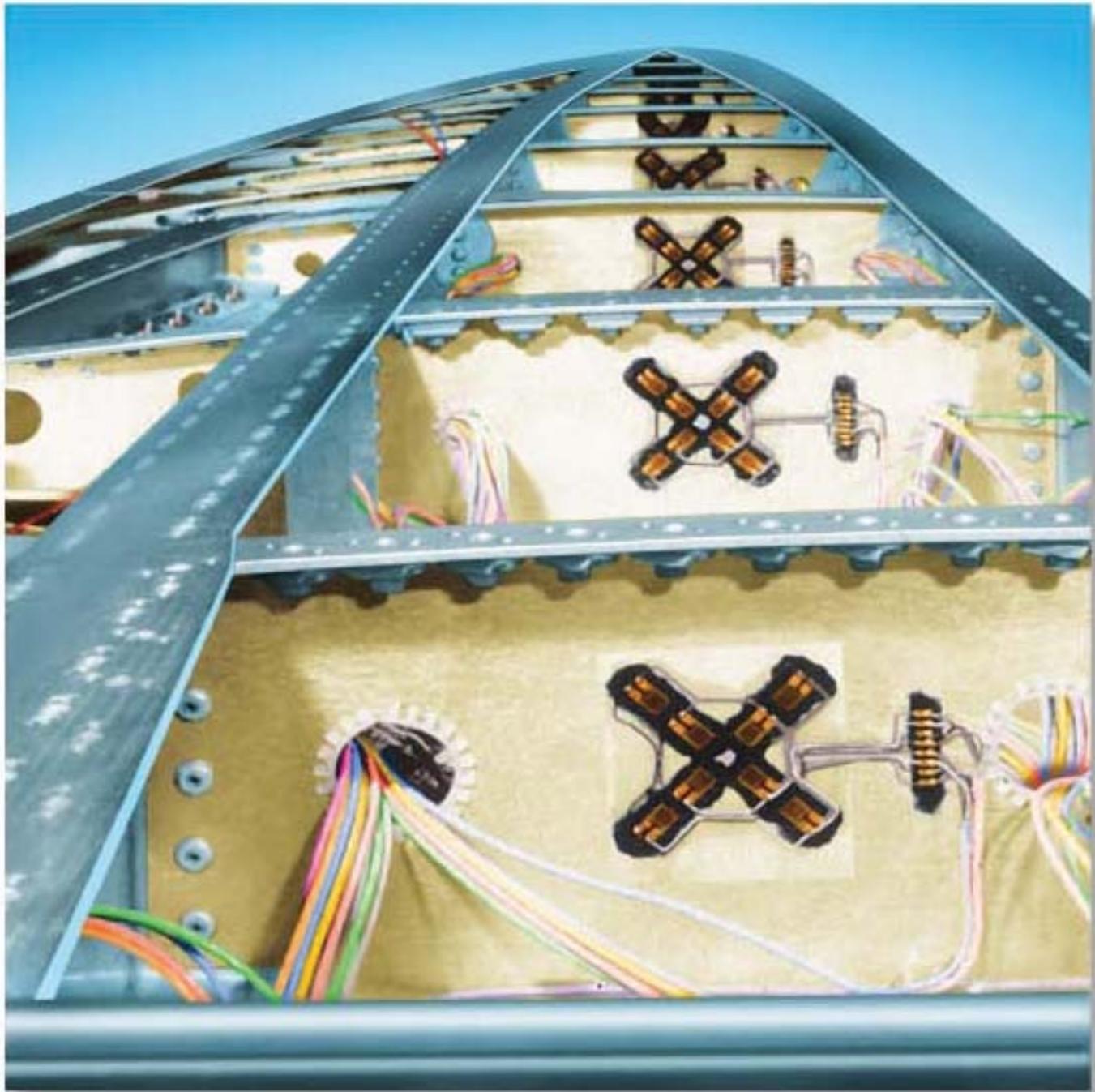
Complex stresses developed within this airplane wing are analyzed from strain gauge data. (Courtesy of Measurements Group, Inc., Raleigh, North Carolina, 27611, USA.)
