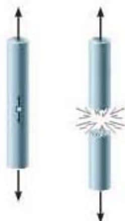
Failure of a brittle material in tension
