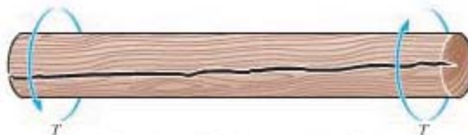
Failure of a wooden shaft due to torsion.
