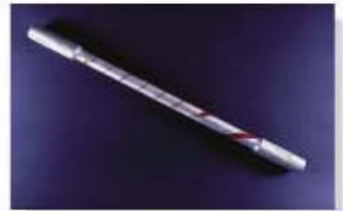
Severe twist of an aluminum specimen caused by the application of a plastic torque.
