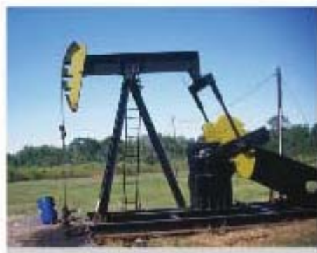
Engineers must account for possible fatigue failure of the moving parts of this oil-pumping rig.
