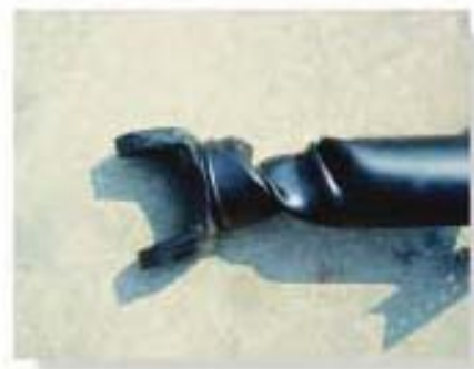
This tubular drive shaft for a truck was subjected to an excessive torque, resulting in failure caused by yielding of the material.
