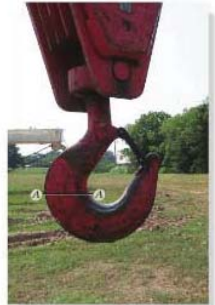
This crane hook represents a typical example of a curved beam.
