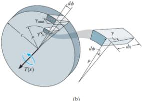
For constant torque and cross-sectional area:
