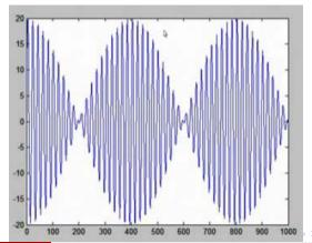
The two Frequencies are predominant here the carrier frequency and the modulated signal.
