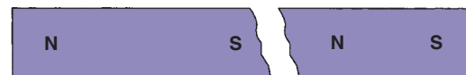
FIGURE 47-2 If a magnet breaks or is cracked, it becomes two weaker magnets.
