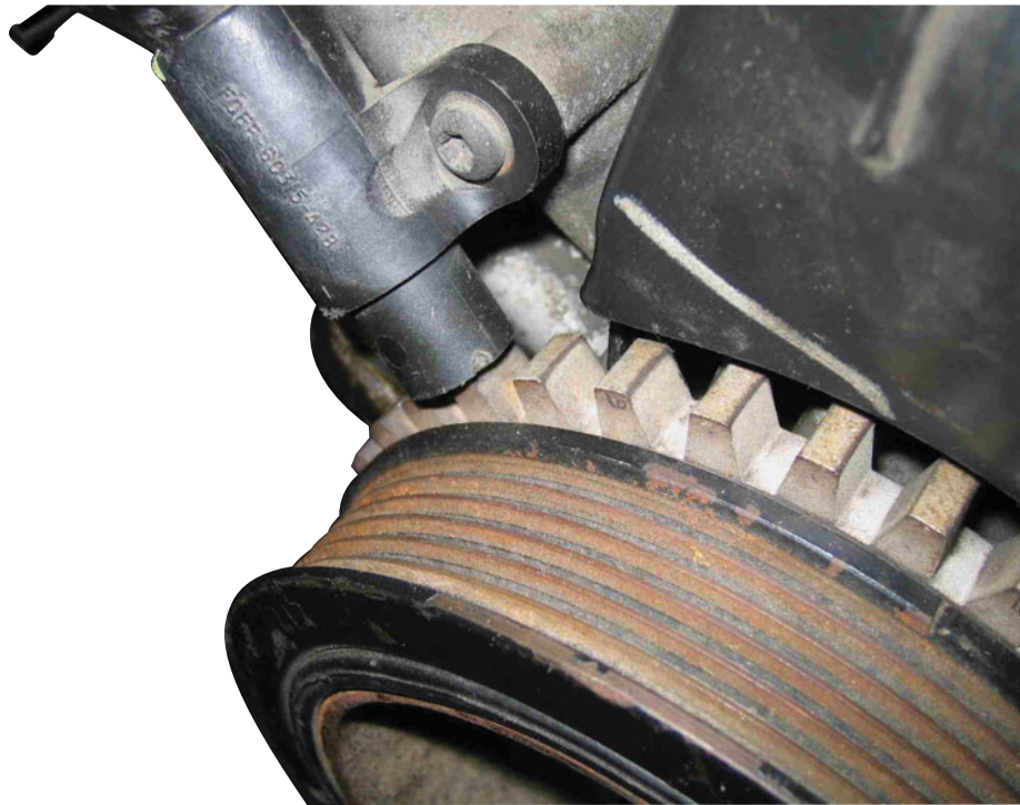
FIGURE 47-6 A crankshaft position sensor and reluctor (notched wheel).
