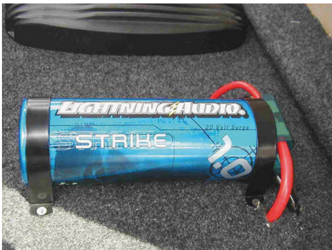
FIGURE 46-9 A 1 farad capacitor used to boost the power to large speakers.
