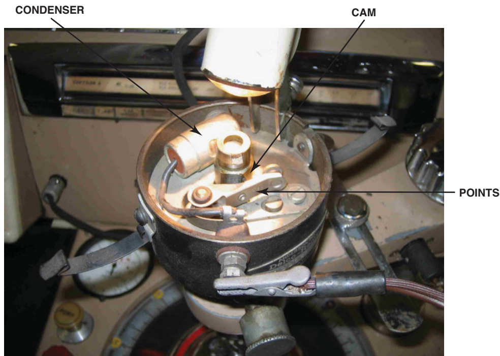
FIGURE 46-7 A point-type distributor shown with the condenser from an old vehicle being tested on a distributor machine.
