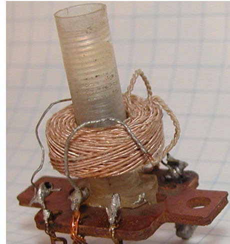
Fig. 14.1.3: Example of a cross-wound coil
