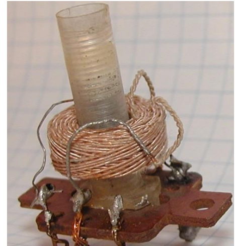
Fig. 11.1.3: Example of a cross-wound coil
