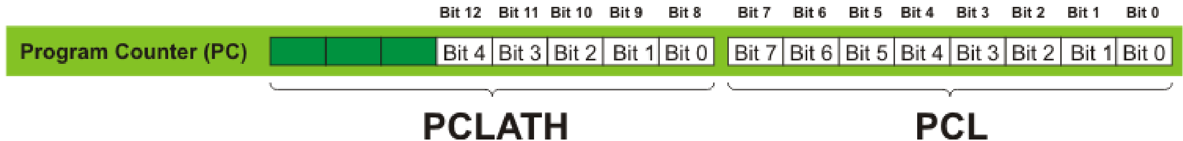
Fig. 2-16 PCL and PCLATH Registers
