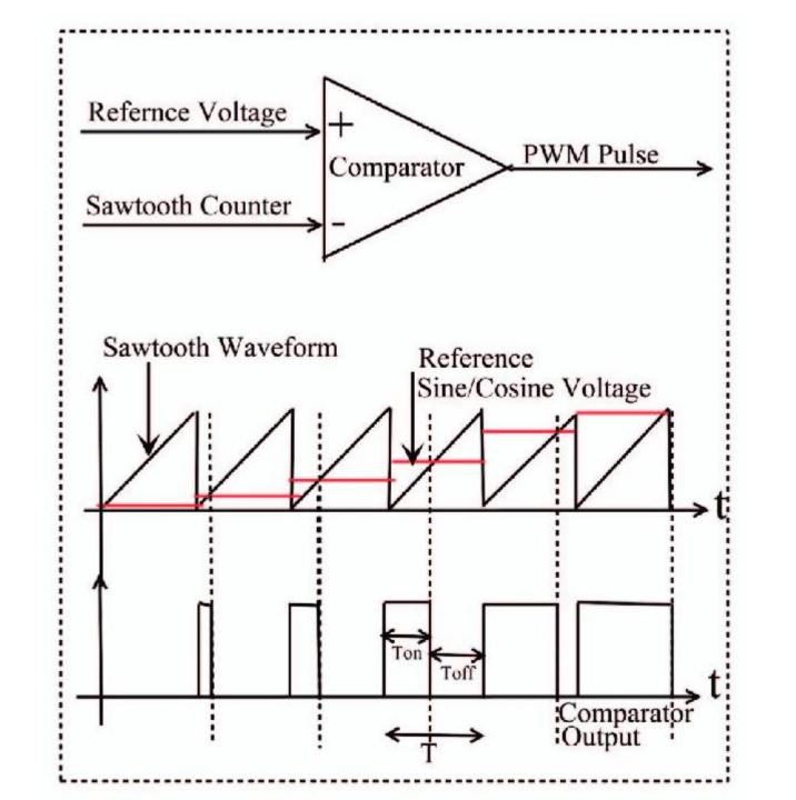
Below diagram shows the PIC16f877a PWM block diagram and output signal generation.
