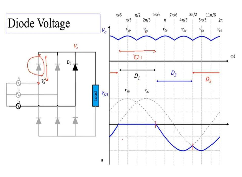
$$v_{avg} = \frac{6}{2\pi} \int_{\pi/6}^{\pi/2} \frac{V_{mL} \sin(\omega t + 30) d\omega t}{V_{ml} \sin(\omega t)} d\omega t$$
