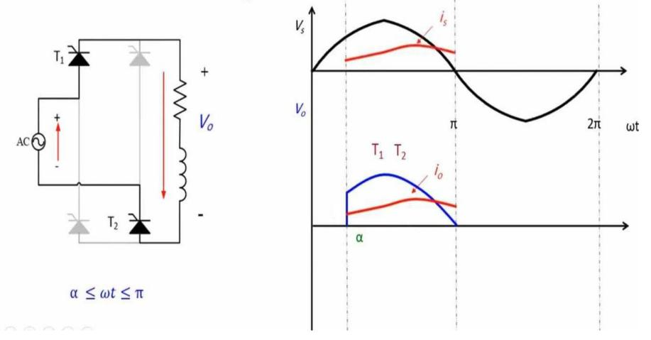
RL Load with Free-Wheeling Diode
