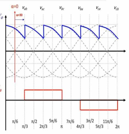
$$v_{avg} = \frac{3}{\pi} \int_{\frac{\pi}{3} + \alpha}^{2\pi/3 + \alpha} V_{mL} \sin(\omega t) d\omega t = \frac{3V_{mL}}{\pi} \cos(\alpha)$$
