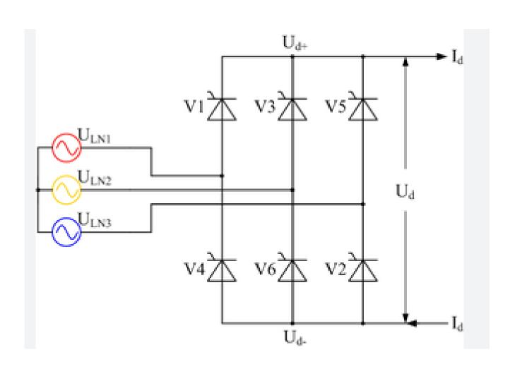
$$v_{avg} = \frac{3}{\pi} \int_{\frac{\pi}{3} + \alpha}^{2\pi/3 + \alpha} V_{mL} \sin(\omega t) d\omega t = \frac{3V_{mL}}{\pi} \cos(\alpha)$$
