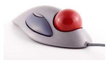
Since the whole device is not moved, a track ball requires less space than a mouse. A track ball comes in various shapes like a ball, a button, or a square.
