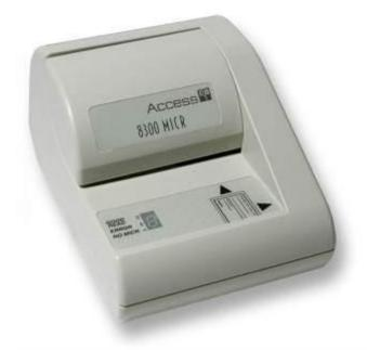
This reading process is called Magnetic Ink Character Recognition (MICR). The main advantages of MICR is that it is fast and less error.
