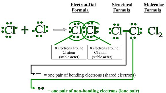
NOTE: There are 3 non-bonding electron pairs (lone pairs) around each Cl atom.
