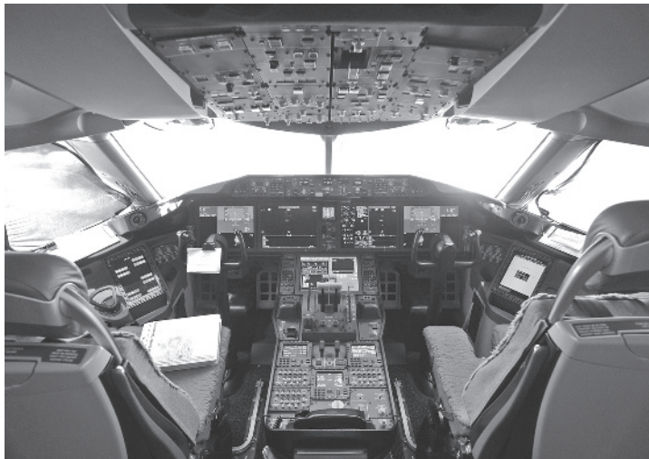
FIGURE 13.3 The flight deck of the Boeing 787 Dreamliner features digital control electronics. The aircraft is equipped with a complete suite of navigation and communication avionics. (Courtesy of Craig F. Walker/Getty Images.)
