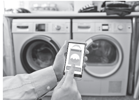
FIGURE DP1.3 Using a smart phone to remotely monitor and control a washing machine. (Photo courtesy of Mikkel William/E+/Getty Images.)
