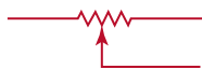
FIGURE 45-16 A rheostat uses only two wires—one is connected to a voltage source and the other is attached to the movable arm.
