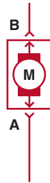
FIGURE 45-14 An electric motor symbol shows a circle with the letter M in the center and two black sections that represent the brushes of the motor. This symbol is used even though the motor is a brushless design.
