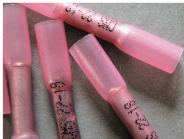
FIGURE 44-23 A typical crimp-and-seal connector. This type of connector is first lightly crimped to retain the ends of the wires and then it is heated. The tubing shrinks around the wire splice, and thermoplastic glue melts on the inside to provide an effective weather-resistant seal.
