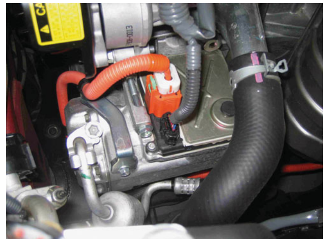
FIGURE 44-27 Always follow the vehicle manufacturer's instructions which include the use of linesman's (high-voltage) gloves if working on circuits that are covered in orange conduit.
