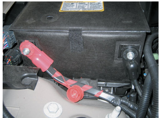
FIGURE 44-2 Battery cables are designed to carry heavy starter current and are therefore usually 4 gauge or larger wire. Note that this battery has a thermal blanket covering to help protect the battery from high underhood temperatures. The wiring is also covered with plastic conduit called split-loom tubing.
