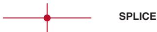
FIGURE 45-9 Two wires that cross at the dot indicate that the two are electrically connected.
