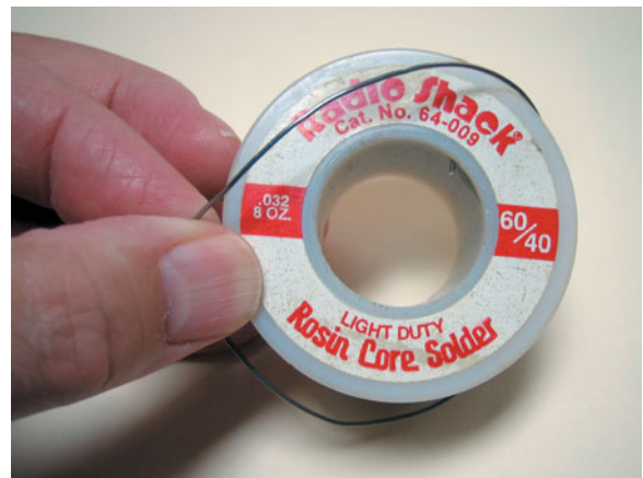
FIGURE 44-18 Always use rosin-core solder for electrical or electronic soldering. Also, use small-diameter solder for small soldering irons. Use large-diameter solder only for large-diameter (large-gauge) wire and higher-wattage soldering irons (guns).
