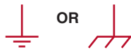
FIGURE 45-6 The ground symbol on the left represents earth ground. The ground symbol on the right represents a chassis ground.
