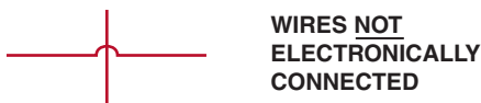
FIGURE 45-10 Wires that cross, but do not electrically contact each other, are shown with one wire bridging over the other.
