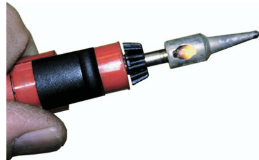
FIGURE 44-19 A butane-powered soldering tool. The cap has a built-in striker to light a converter in the tip of the tool. This handy soldering tool produces the equivalent of 60 watts of heat. It operates for about 1/2 hour on one charge from a commonly available butane refill dispenser.
