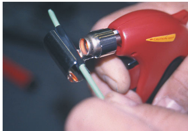
FIGURE 44-22 A butane torch especially designed for use on heat shrink applies heat without an open flame, which could cause damage.
