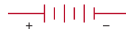
FIGURE 45-5 The symbol for a battery. The positive plate of a battery is represented by the longer line and the negative plate by the shorter line. The voltage of the battery is usually stated next to the symbol.
