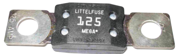
FIGURE 44-13 A 125 ampere rated mega fuse used to control the current from the alternator.
