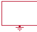
FIGURE 45-21 This symbol represents a component that is case grounded.
