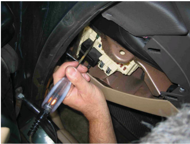
FIGURE 44-7 To test a fuse, use a test light to check for power at the power side of the fuse. The ignition switch and lights may have to be on before some fuses receive power. If the fuse is good, the test light should light on both sides (power side and load side) of the fuse.
