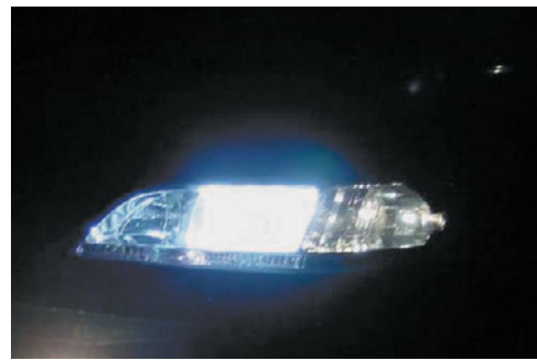
FIGURE 56-20 HID (xenon) headlights emit a whiter light than halogen headlights and usually look blue compared to halogen bulbs.
