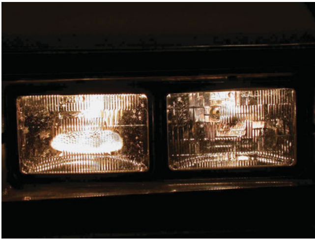
FIGURE 56-16 A typical four-headlight system using sealed beam headlights.
