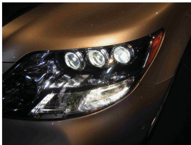
FIGURE 56-21 LED headlights usually require multiple units to provide the needed light as seen on this Lexus LS600h.
