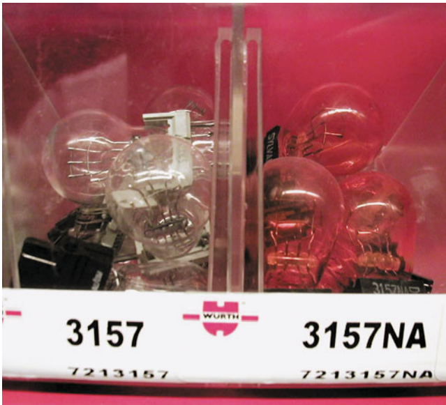
FIGURE 56-2 Bulbs that have the same trade number have the same operating voltage and wattage. The NA means that the bulb uses a natural amber glass ampoule with clear turn signal lenses.
