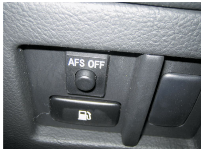
FIGURE 56-26 Typical dash-mounted switch that allows the driver to disable the front lighting system.
