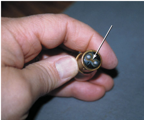
FIGURE 56-4 Corrosion caused the two terminals of this dual-filament bulb to be electrically connected.
