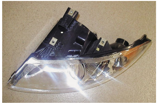
FIGURE 56-17 A typical composite headlamp assembly. The lens, housing, and bulb sockets are usually included as a complete assembly.
