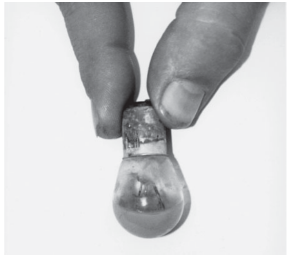
FIGURE 56-5 Often the best diagnosis is a thorough visual inspection. This bulb was found to be filled with water, which caused weird problems.
