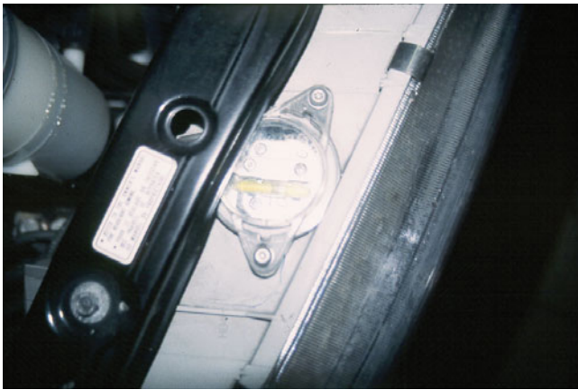
FIGURE 56-23 Many composite headlights have a built-in bubble level to make aiming easy and accurate.
