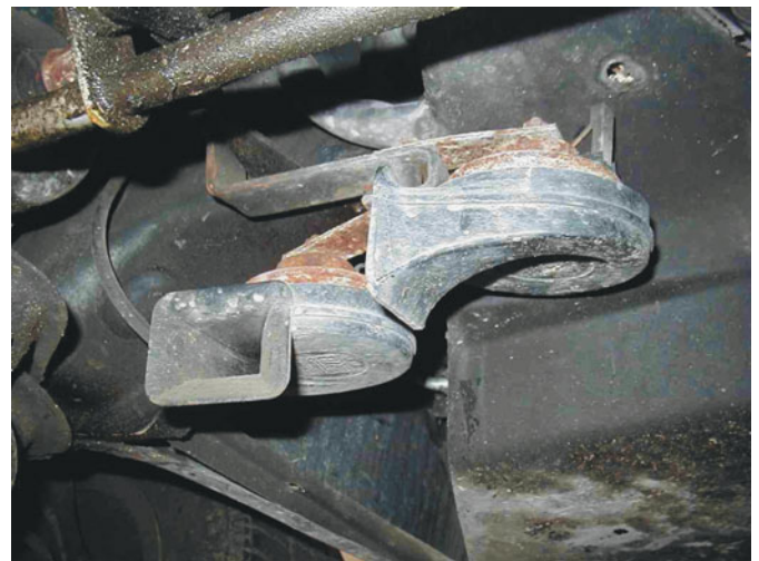
FIGURE 58-1 Two horns are used on this vehicle. Many vehicles use only one horn, often hidden underneath the vehicle.
