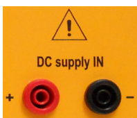
2.1-10 Power supply connectors of the module. Voltage must be between 10V and 35V.
