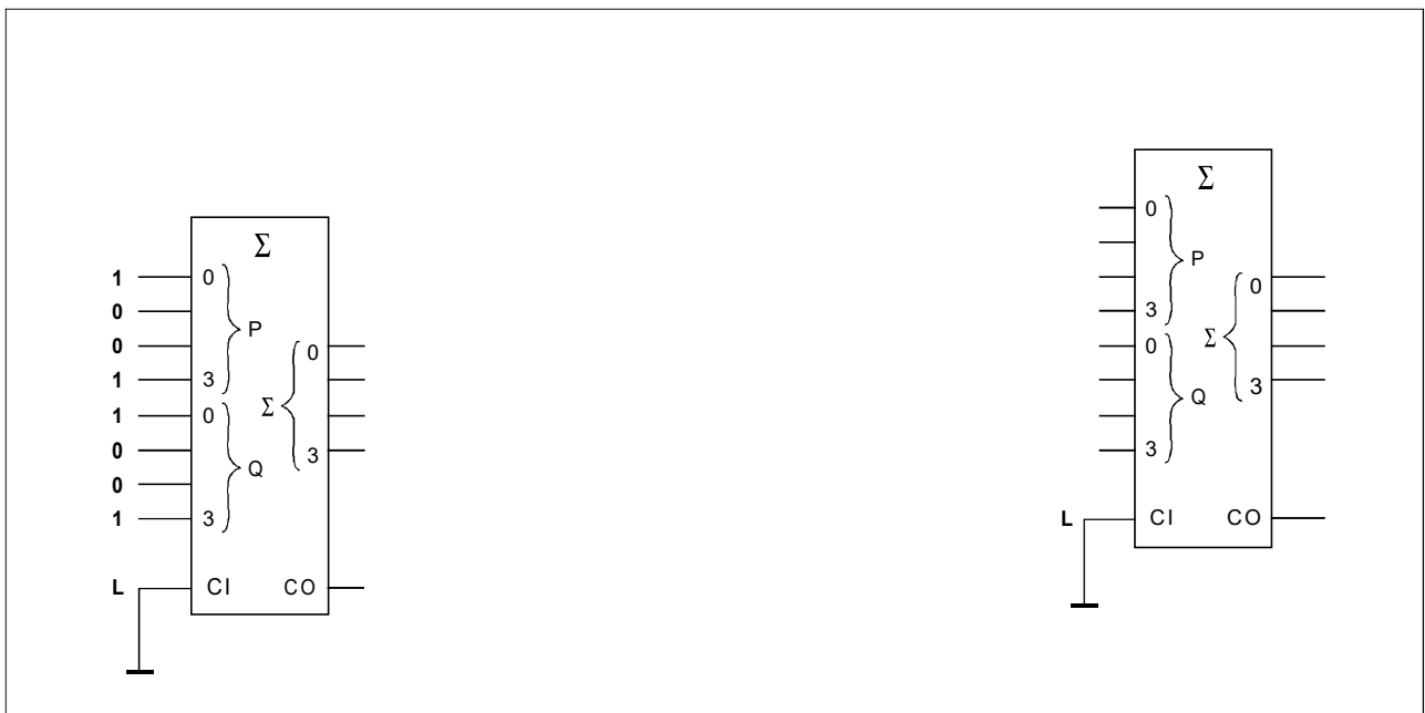
Fig. 6.2.3.7 Simplified correction circuit
