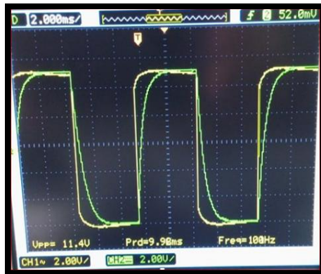
Fig. 4: Output voltage of integrator circuit at different time constant.
