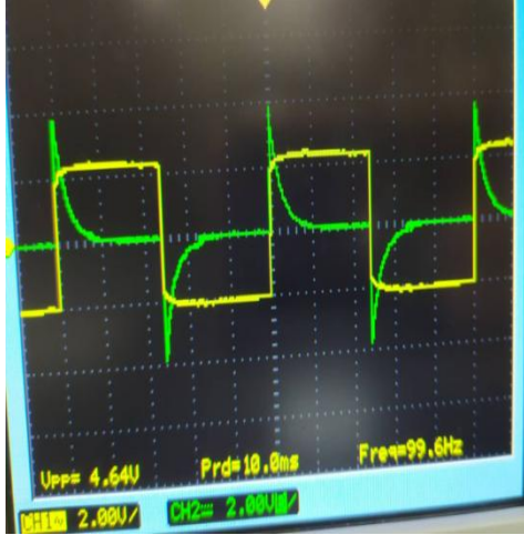
Fig. 7: Output voltage of differentiator circuit at different time constant obtained in lab.
