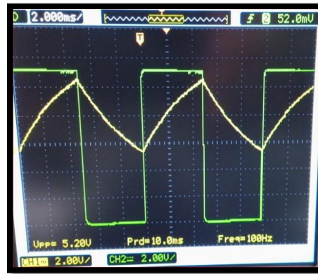
Fig. 4: Output voltage of integrator circuit at different time constant.
