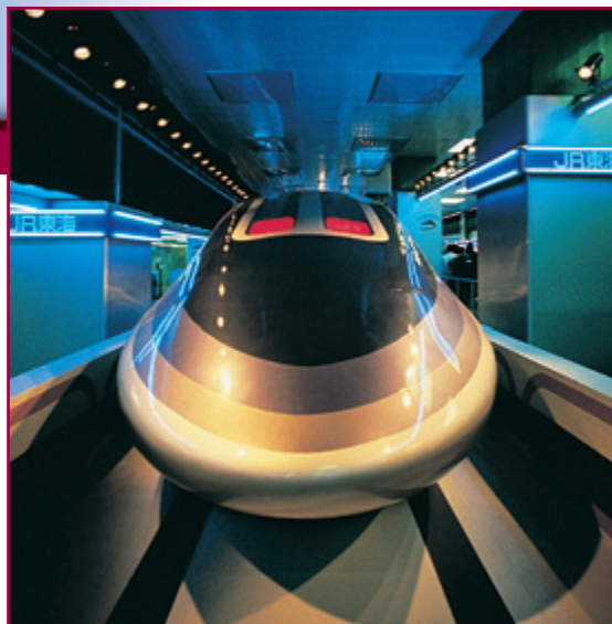
This express train in Tokyo, Japan, which utilizes the Meissner effect, levitates above the track and can reach speeds exceeding 225 km/h.
