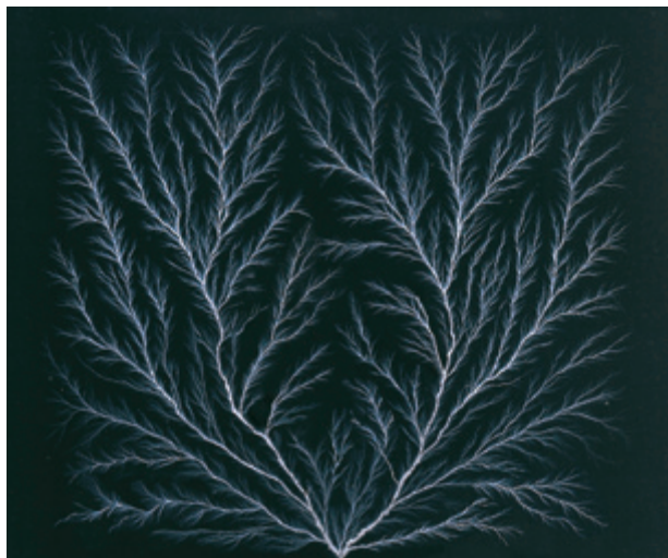
Figure 8 The markings caused by electrical breakdown in this material look similar to the lightning bolts produced when air undergoes electrical breakdown.
