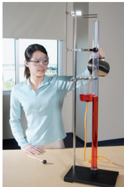
Figure 1 Step 7: From the position of greatest resonance, move the reservoir up 2 cm and down again until you find the exact position.
