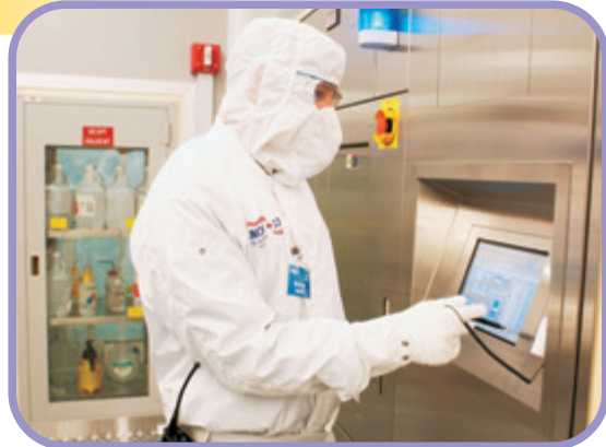
Brad Baker is creating a recipe on the plasma etch tool to test a new process.
