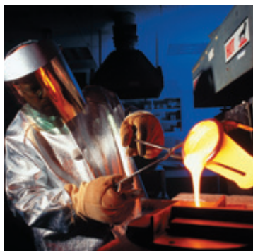
Figure 1 This molten metal has a bright yellow glow because of its high temperature.
