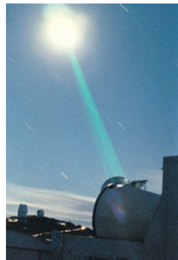
Figure 25 A laser beam is fired at reflectors on the moon, which is more than 380 000 km away.
