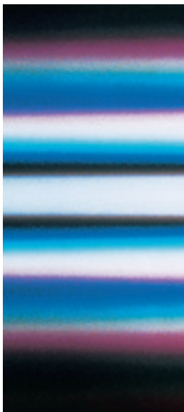
Figure 5 When waves of white light from two coherent sources interfere, the pattern is indistinct because different colors interfere constructively and destructively at different positions.
