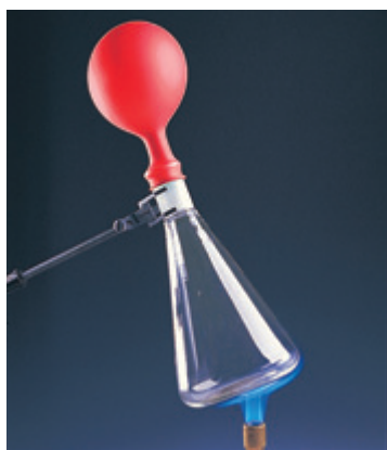
Figure 1 Energy transferred as heat turns water into steam. Energy from the steam does work on the air outside the balloon.
