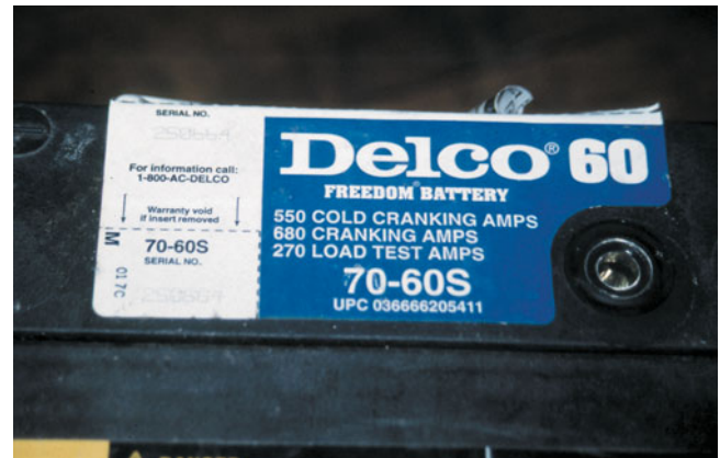
FIGURE 51-6 This battery has cold-cranking amperes (CCA) of 550 A, cranking amperes (CA) of 680 A, and load test amperes of 270 A listed on the top label. Not all batteries have this complete information.
