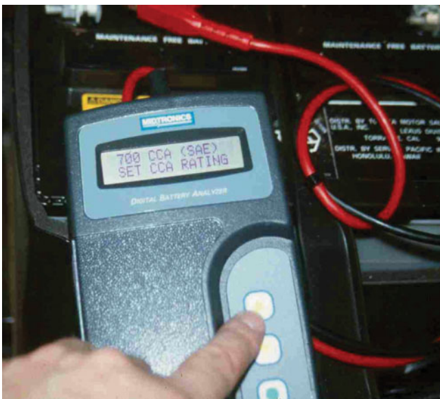
FIGURE 51-10 A conductance tester is very easy to use and has proved to accurately determine battery condition if the connections are properly made. Follow the instructions on the display exactly for best results.
