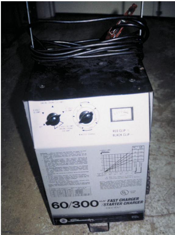
FIGURE 51-11 A typical industrial battery charger. Be sure that the ignition switch is in the off position before connecting any battery charger. Connect the cables of the charger to the battery before plugging the charger into the outlet. This helps prevent a voltage spike and spark that could occur if the charger happened to be accidentally left on. Always follow the battery charger manufacturer's instructions.
