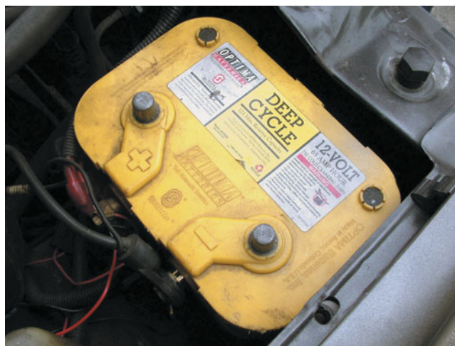
FIGURE 50-9 An absorbed glass mat battery is totally sealed and is more vibration resistant than conventional lead-acid batteries.
