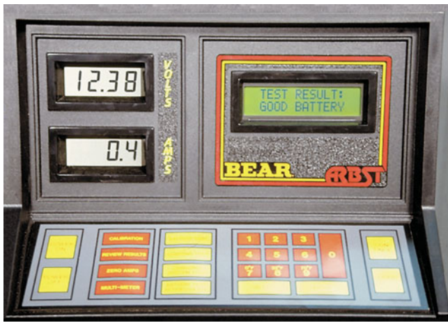
FIGURE 51-7 An alternator regulator battery starter tester (ARBST) automatically loads the battery with a fixed load for 15 sec. to remove the surface charge, then removes the load for 30 sec. to allow the battery to recover, and then reapplies the load for another 15 sec. The results of the test are then displayed.
