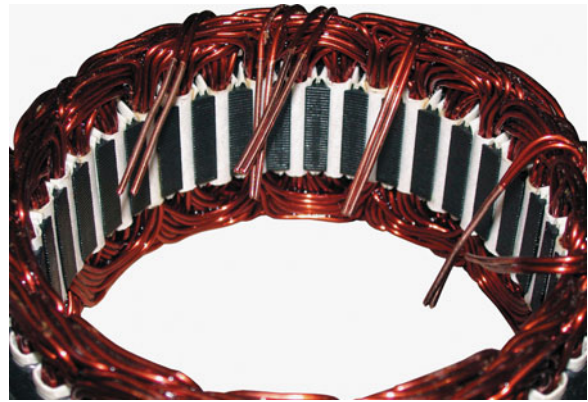
FIGURE 54-16 A stator assembly with six, rather than the normal three, windings.
