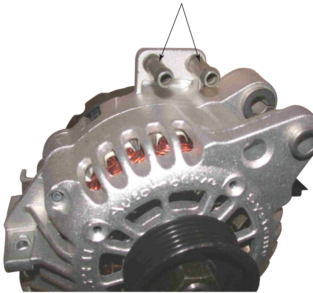
FIGURE 54-20 A coolant-cooled alternator showing the hose connections where coolant from the engine flows through the rear frame of the alternator.
