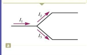
The amount of water flowing out of the branches on the right must equal the amount flowing into the single branch on the left.
