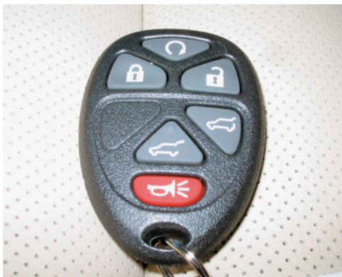
FIGURE 52-5 The top button on this key fob is the remote start button.
