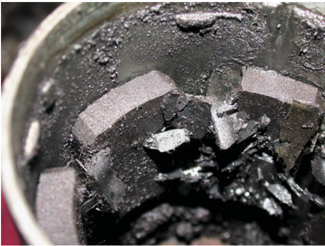
FIGURE 52-19 This starter permanent magnet field housing was ruined when someone used a hammer on the field housing in an attempt to “fix” a starter that would not work. A total replacement is the only solution in this case.
