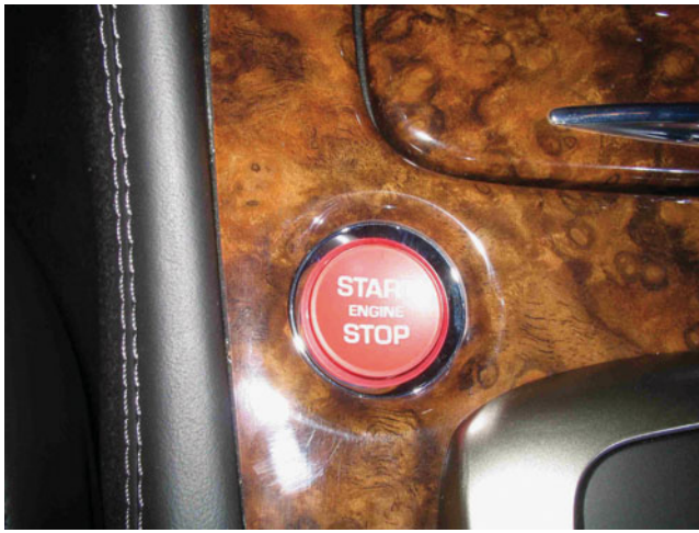
FIGURE 52-4 Instead of using an ignition key to start the engine, some vehicles are using a start button which is also used to stop the engine, as shown on this Jaguar.
