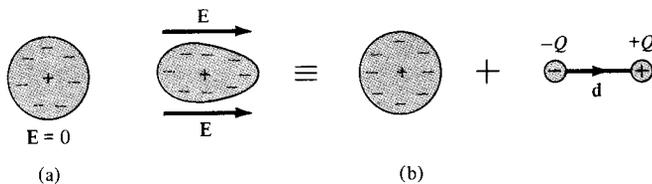
Figure 5.6 Polarization of a nonpolar atom or molecule.
