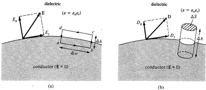
Figure 5.12 Conductor–dielectric boundary.
