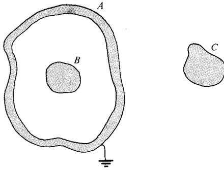
Figure 5.13 Electrostatic screening.
