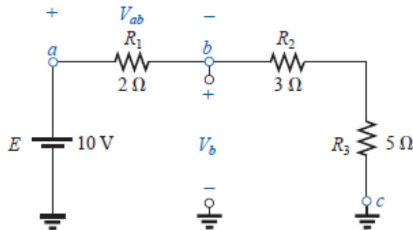
**EXAMPLE** Design the voltage divider of Fig. such that  $V_{R_1} = 4V_{R_2}$ .
