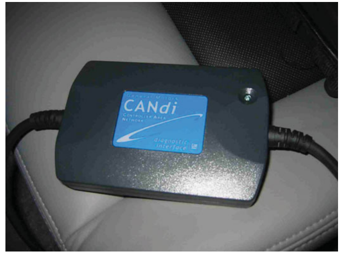
FIGURE 49-12 A CANdi module will flash the green LED rapidly if communication is detected.
