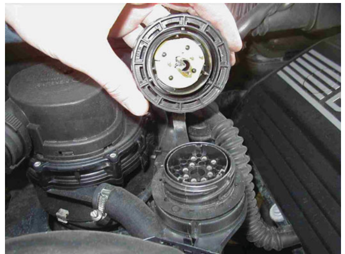
FIGURE 49-23 A typical 38-cavity diagnostic connector as found on many BMW and Mercedes vehicles under the hood. The use of a breakout box (BOB) connected to this connector can often be used to gain access to module BUS information.
