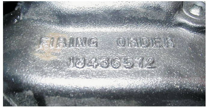
FIGURE 69-12 The firing order is cast or stamped on the intake manifold on most engines that have a distributor ignition.
