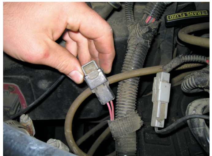
FIGURE 69-22 A SPOUT connector on a Ford that is equipped with a distributor ignition. This connector has to be disconnected to separate the PCM in order to set base ignition timing.
