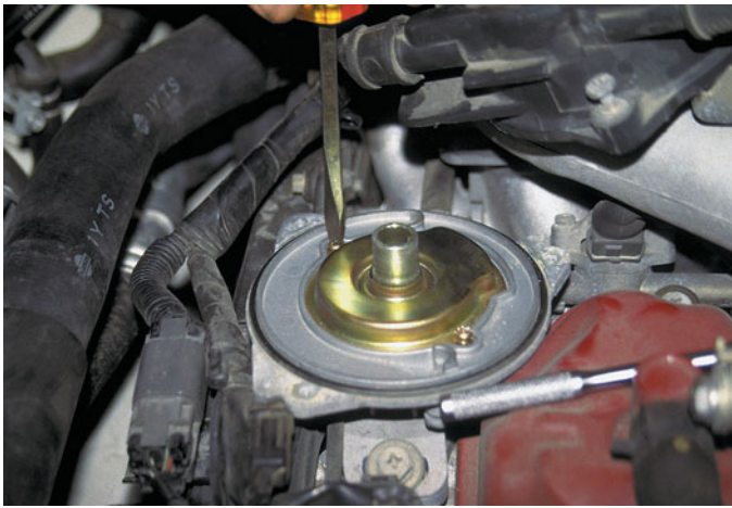
FIGURE 69-11 A light shield being installed before the rotor is attached.
