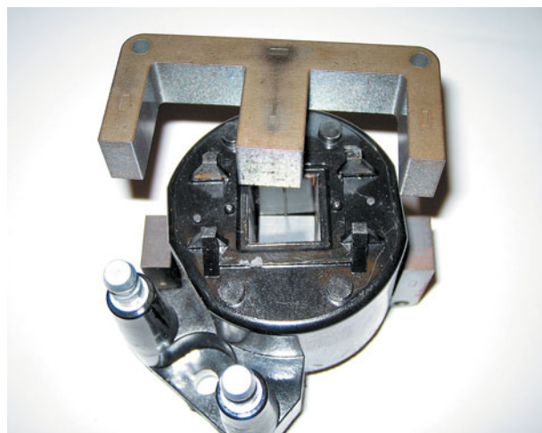
FIGURE 69-3 The steel laminations used in an E coil help increase the magnetic field strength, which helps the coil produce higher energy output for a more complete combustion in the cylinders.
