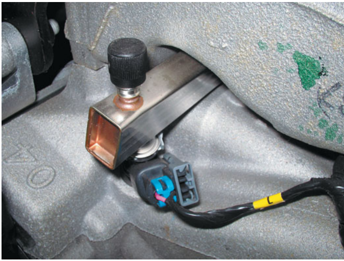
FIGURE 78-15 A rectangular-shaped fuel rail is used to help dampen fuel system pulsations and noise caused by the injectors opening and closing.
