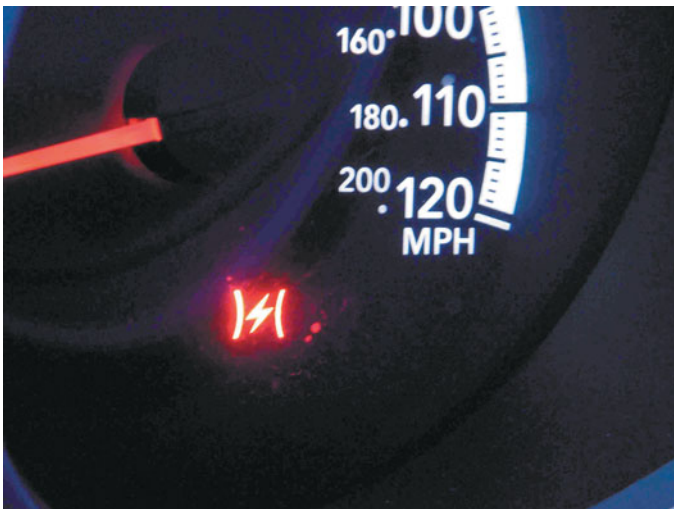
FIGURE 80-10 A symbol used on a Chrysler vehicle indicating a fault with the electronic throttle control.
