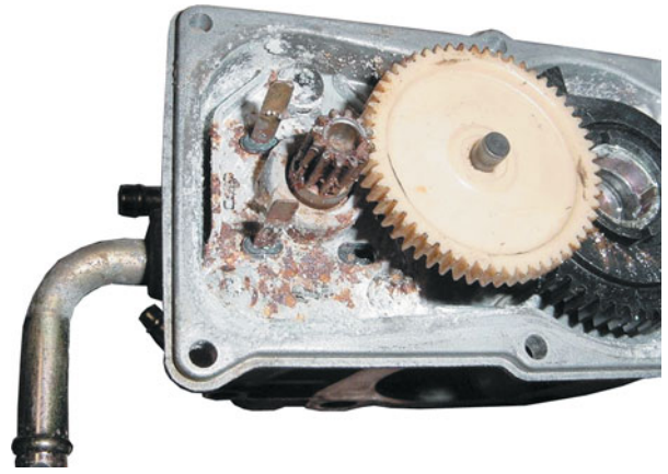
FIGURE 80-12 A corroded electronic throttle control assembly shown with the cover removed.
