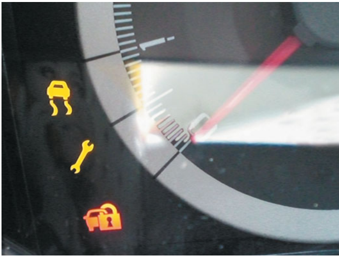
FIGURE 80-9 A wrench symbol warning lamp on a Ford vehicle. The symbol can also be green.
