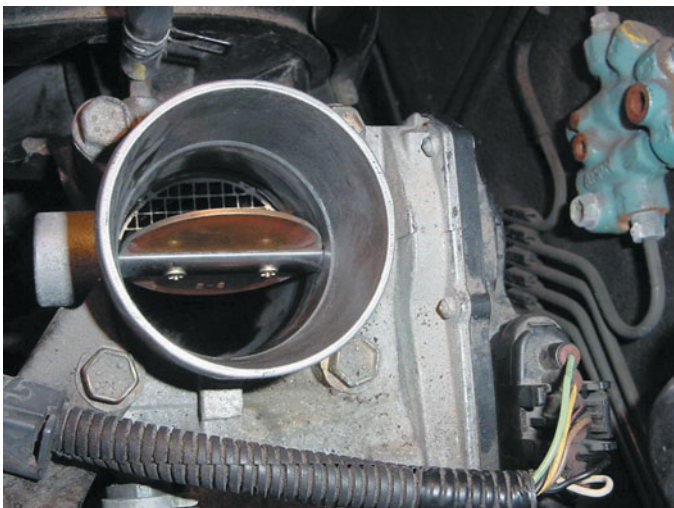
FIGURE 80-11 The throttle plate stayed where it was moved, which indicates that there is a problem with the electronic throttle body control assembly.
