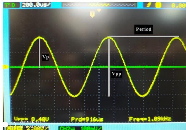
Fig. 6: Oscilloscope diagram of a sinusoidal signal.
