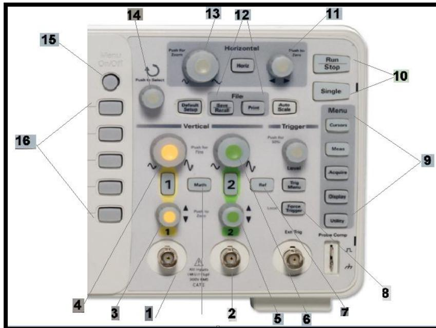
Fig. 2: Front view of the control units of the digital oscilloscope (DSO1052B).
