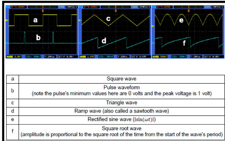
Fig. 5: Some examples of Non-sinusoidal wave.
