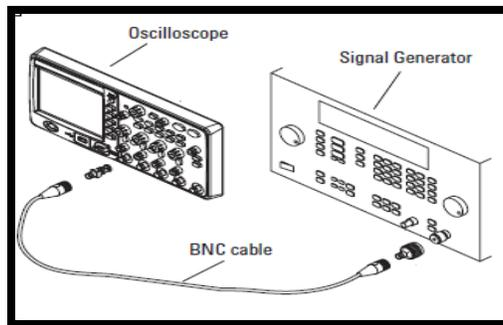
Fig. 9: Oscilloscope connected with signal generator with BNC cable.
