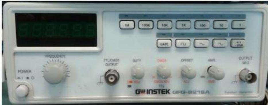
Fig. 3: GFG-8250A Function Generator.
