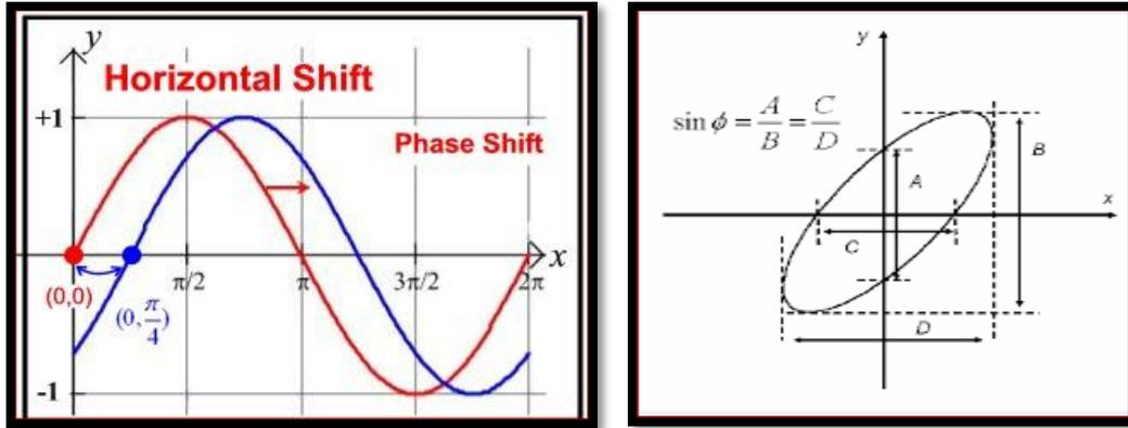
Fig. 8: The phase difference between two signals of the same frequency with the Lissajous method.
