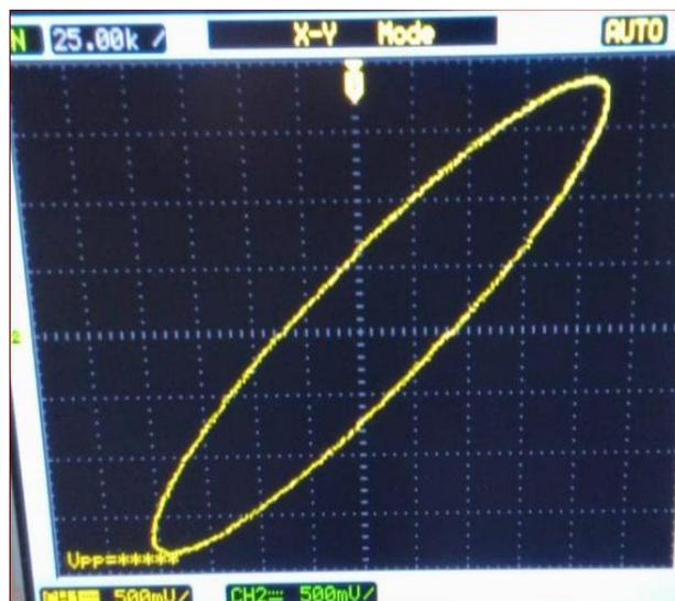
Fig. 7: Oscilloscope diagram of XY time mode.
