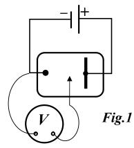
Connect the points of equal voltage (potential) with a smooth line and label them. These are equipotential surfaces.
