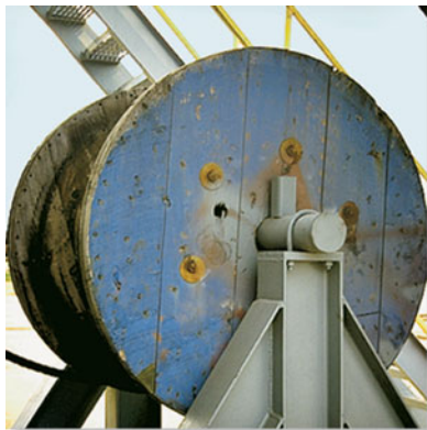
Unwinding the cable from this spool requires overcoming friction from the supporting shaft.
